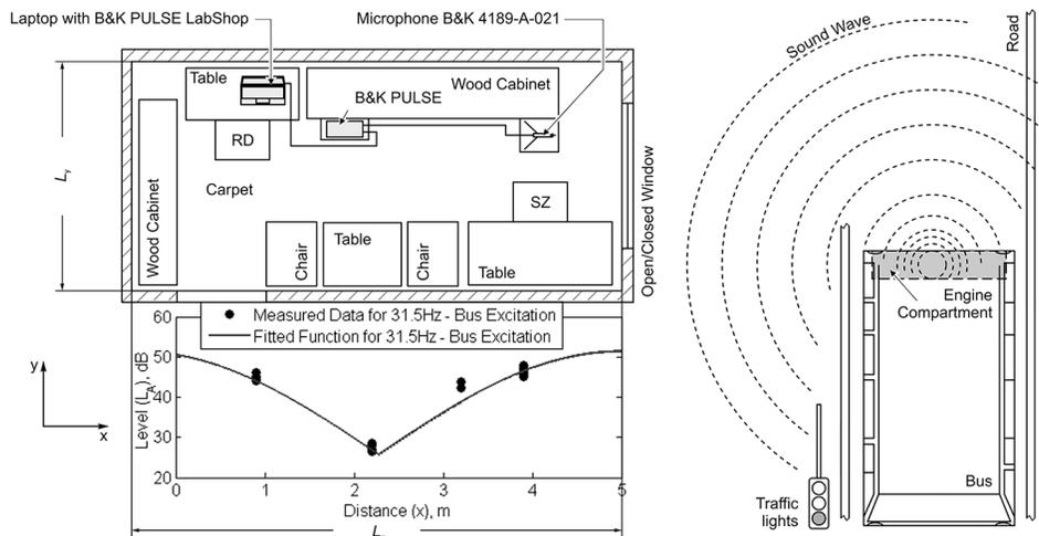
Figure 1: Measurement set-up with results plotted for bus excitation (SOR B 9.5)
