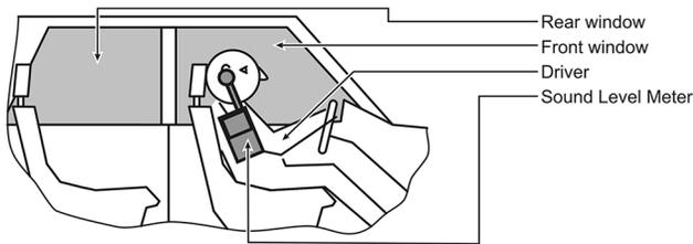
Figure 6: Schematics of the measurement set-up inside a passenger car while driving
