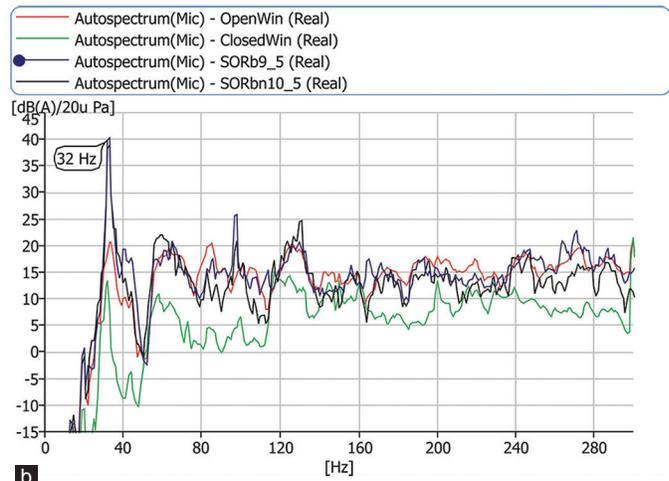
Figure 2: First two modes of the standing wave generated in the office by loudspeaker (a) axial mode (1, 0, 0) and (b) axial mode (2, 0, 0)
