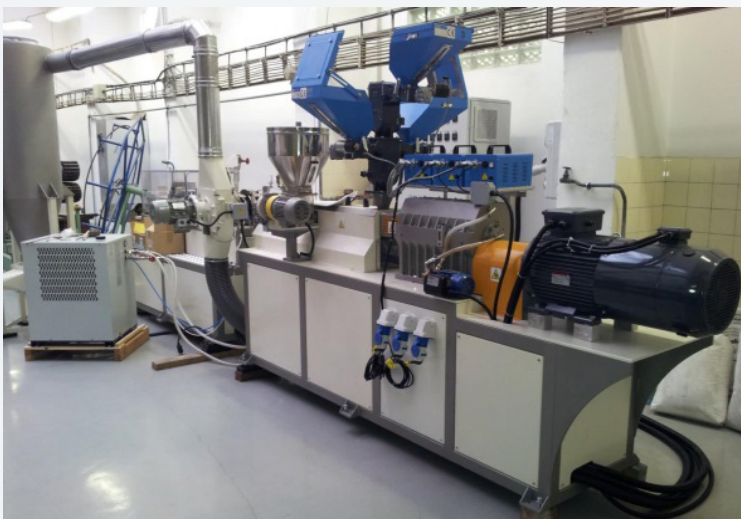
Extruder with granulator and cooler features
