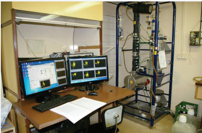
Distillation column - Armfield UOP3CC
