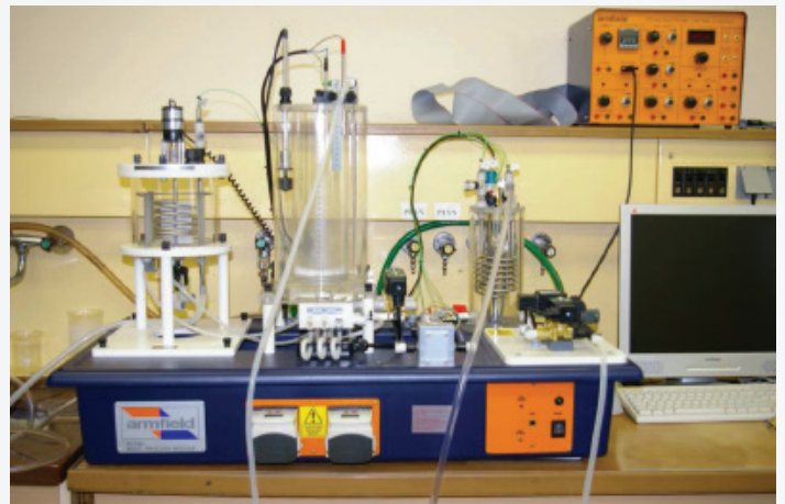
Multifunction station Armfield PCT40
