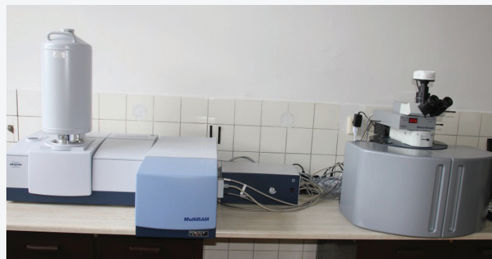
Ramanov spektrometer MultiRAM s mikroskopom RamScope III
