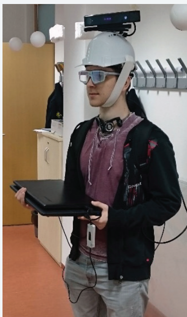
RGB-D data acquisition using Kinect (on helmet). Eye tracker SMI (glasses).
