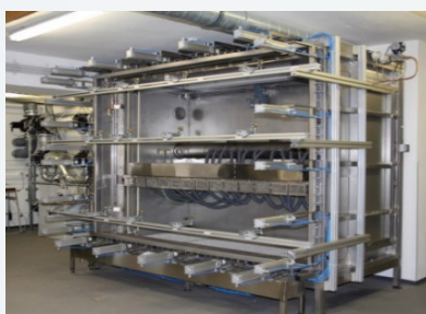
Dažďová komora pre výskum prieniku vody cez detaily stien a striech / Rain chamber for research of penetration of water through details of walls and roofs
