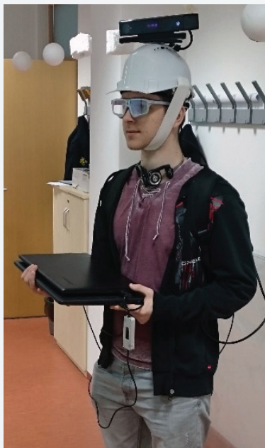
RGB-D data acquisition using Kinect (on helmet). Eye tracker SMI (glasses).
