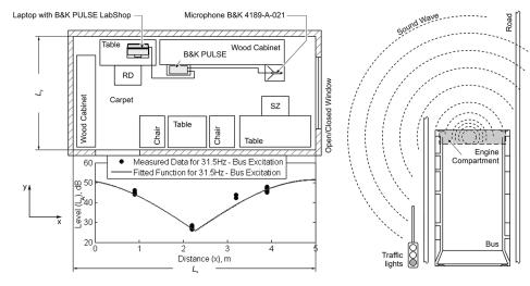
Figure 1: Measurement set-up with results plotted for bus excitation (SOR B 9.5)
