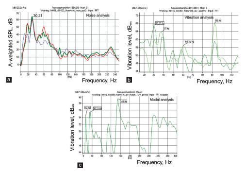
Figure 5: Frequency analysis (a) frequency spectrum of noise in the bedroom, (b) frequency spectrum of the hot-water pipes vibration, and (c) modal analysis of the hot-water pipes
