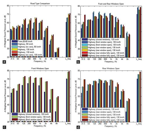
Figure 7: Octave-band analysis: Comparison of measurements (a) for different road types, (b) for rear and front windows open, (c) for front window open, and (d) for rear window open
