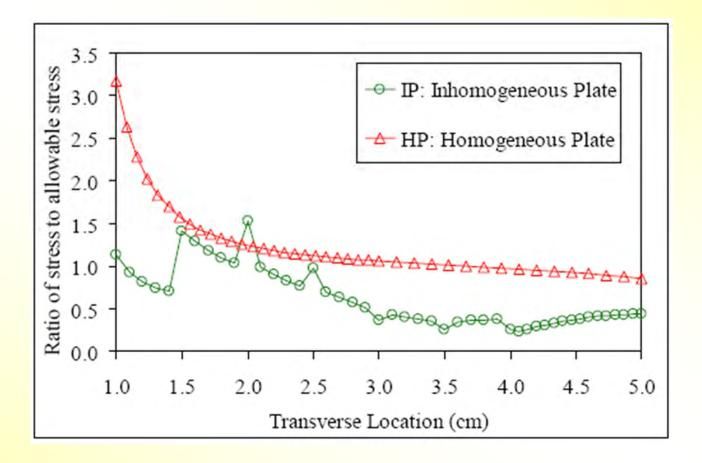
**Stress failure index (load carrying capacity)**
